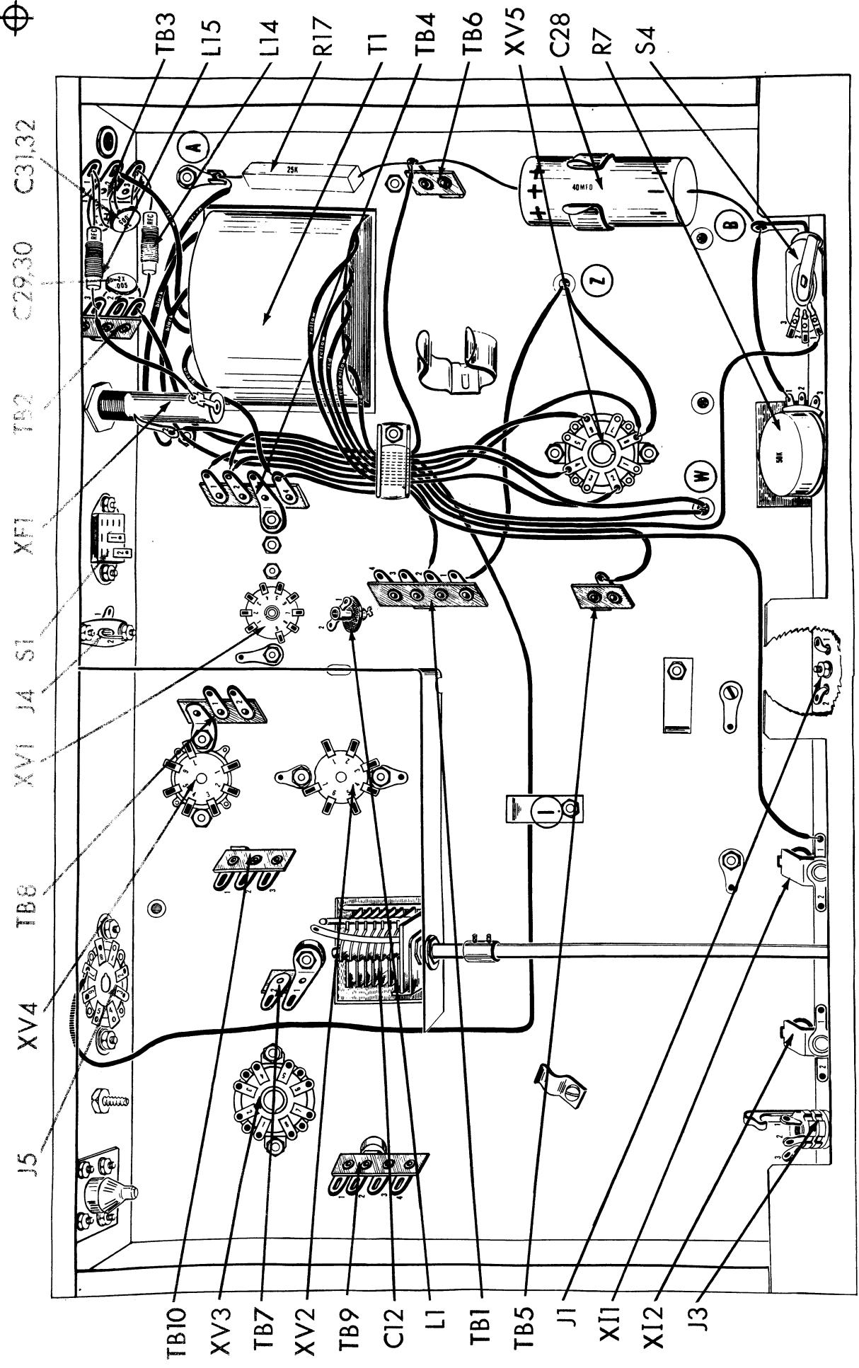
1. (✓) Fig. 4. Connect the shorter of the two leads from hole "Z" to XV5-8 (C) and the longer lead to TB1-1 (C).
